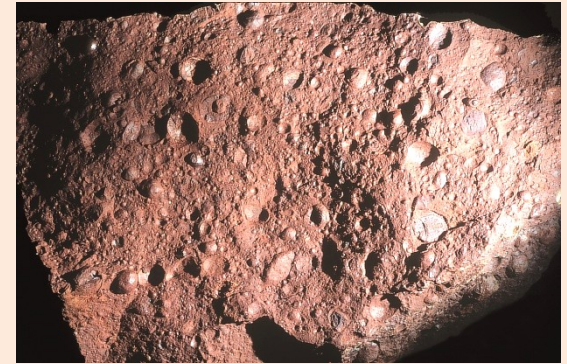
BAUXITE (rock formed from gibbsite, diaspore and boehmite) mix of aluminium hydroxides and oxides Miralles (Anoia) Catalonia
