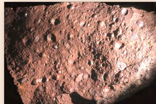
BAUXITE (rock formed from gibbsite, diaspore and boehmite) mix of aluminium hydroxides and oxides Miralles (Anoia) Catalonia
